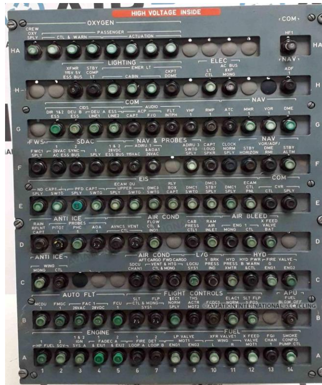
Fig. 4. A330 Secondary Circuit Breaker panel [4]
