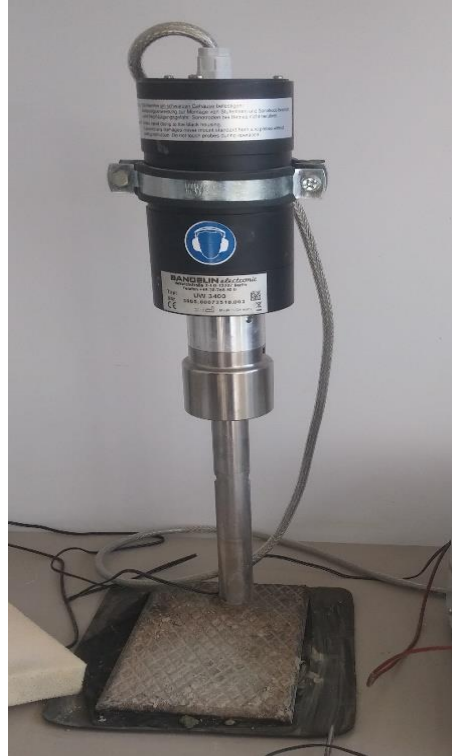
Pav.23 Ultragarsinis dispergatorius Bandelin electronic
