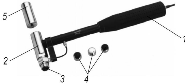
Fig. 1.16 An impact hammer with changeable tips of different hardness [36]: 1 – handle, 2 – impacting mass, 3 – mounted plastic tip, 4 – extra plastic, steel and rubber tips, 5 – additional mass
