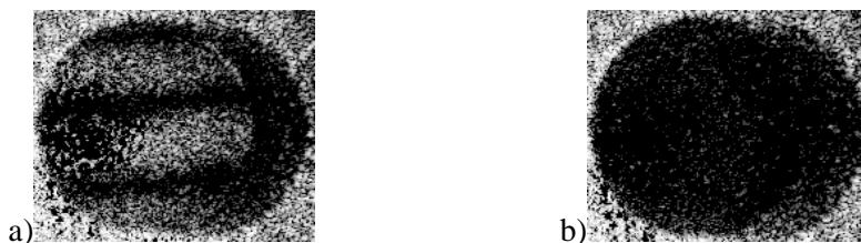
Fig. 3.27. ODS analysis of VAP-2: frequency of 17.750 kHz (a) and 3.1 kHz (b)
