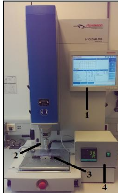
Fig. 2.2. HiQ DIALOG 1200 UHE experimental setup: display (1), UAT (2), anvil with the master mould and a polymer piece on it (3), heating tool (4).
