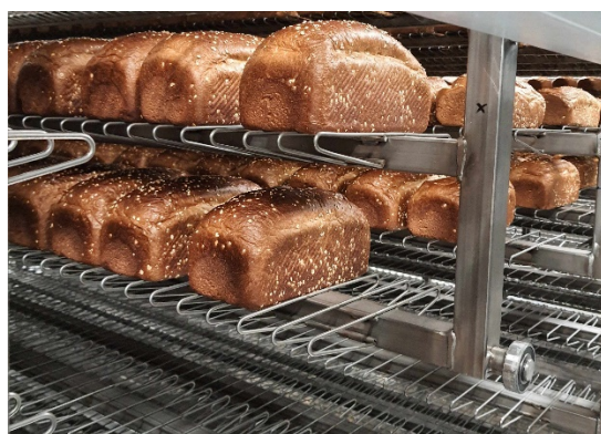
Figure 1. Cooling conveyor hanger with bread
