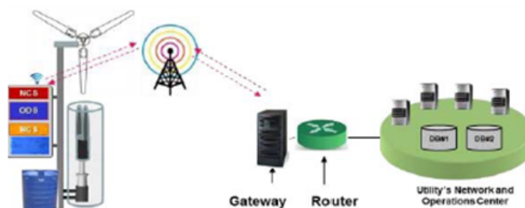
Figure 4. Local network communication subsystem
