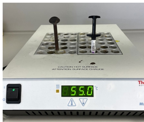
Fig. 1 Pre-heating of the bonding composite in a multi block-heater
