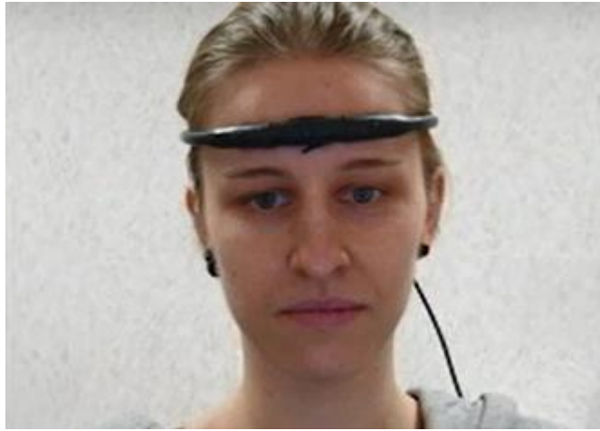
Fig. 10. The test subject with OCZ NIA device
