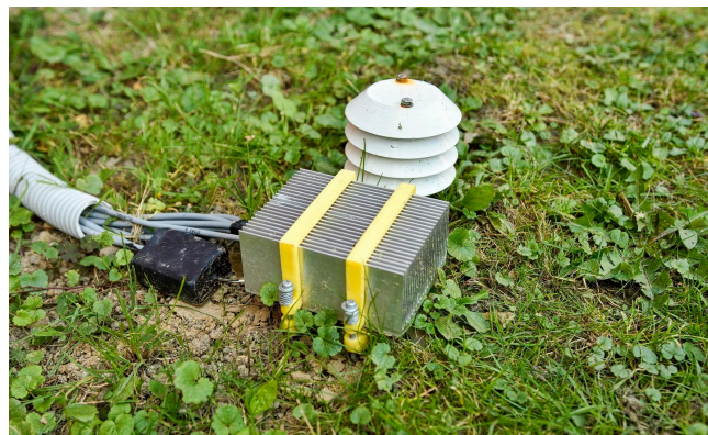
Figure 6. The energy-harvesting device deployed at the experiment site. The upper part of the prototype is shown, with a heat sink and its ambient temperature sensor equipped with a radiation shield.
