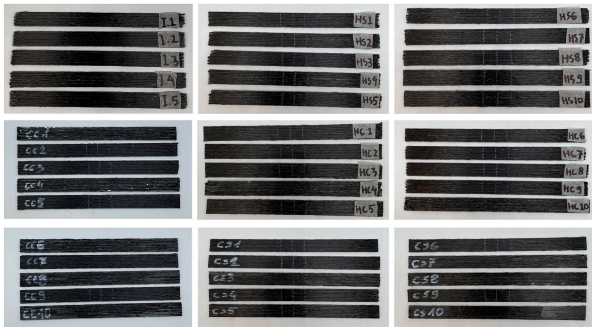
Fig. 1. AM CFRP specimens printed with a modified FDM printer prior to thermal and mechanical testing.
