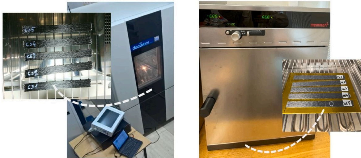
Fig. 3. An automated environmental chamber for cold thermal treatment (left) and an air-circulated oven for hot thermal treatment (right).
