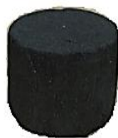
Fig.3 Sample of charcoal material (Thickness 25 mm; diameter 30 mm)
