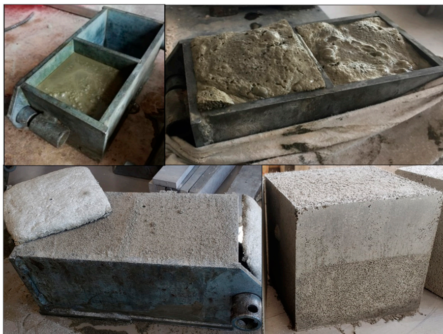
Figure 4. Transformation of the slurry mixture into aluminum-based ultra-lightweight concrete with waste glass powder.
