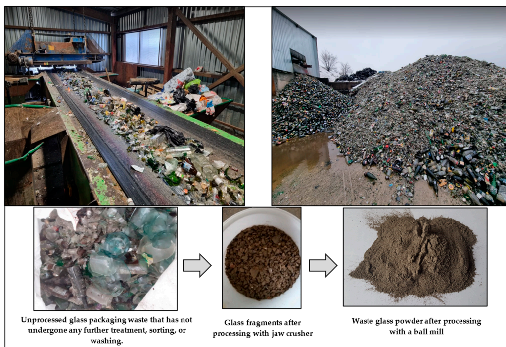
Figure 3. The conversion process of waste glass shards into waste glass powder.
