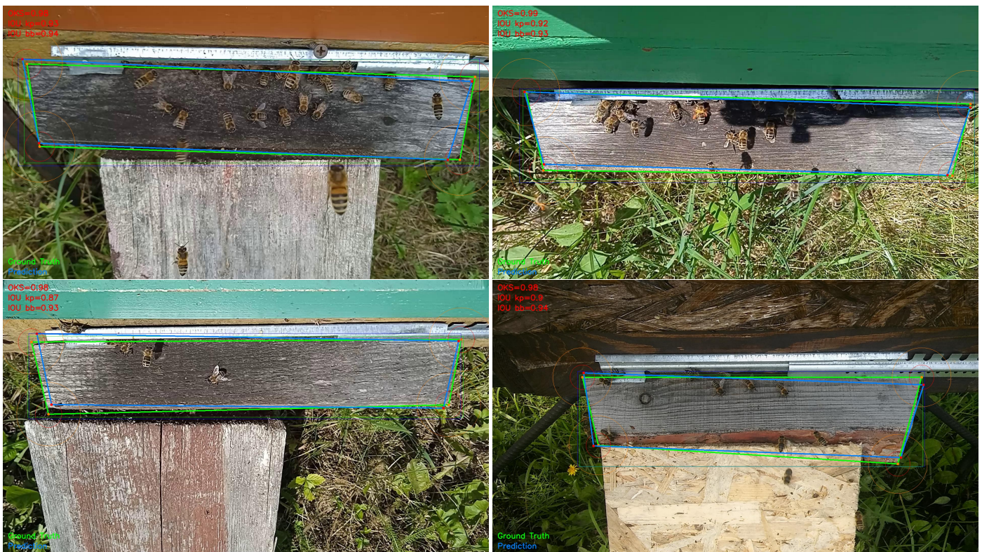
Figure 8. Detected entrance ramps: the ground truth edges are marked in green, while the predicted ramp is marked in blue. Red and orange circles indicate OKS levels of 0.95 and 0.75, respectively, when the standard deviation \sigma = 0.125 is applied to all corners of the ramp.
