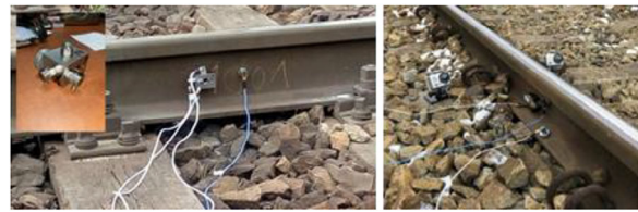
FIGURE 1 The measurement setup showing the vibration sensors mounted on the surface of the rail. Photographs courtesy of Rafal Burdzik.
