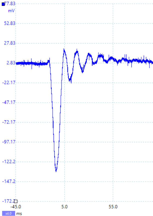
Fig. 11 „Bump“ test results of the first specimen
