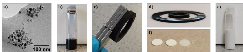
Figure 1: a) TEM image of synthesised \text{CoFe}_2\text{O}_4 nanoparticles. b) Stable UV-curable \text{CoFe}_2\text{O}_4 ink. c-d) Printed \text{CoFe}_2\text{O}_4 samples. e) Stable UV-curable \text{BaTiO}_3 ink. f) Printed samples with decreasing \text{BaTiO}_3 content, from left to right.
