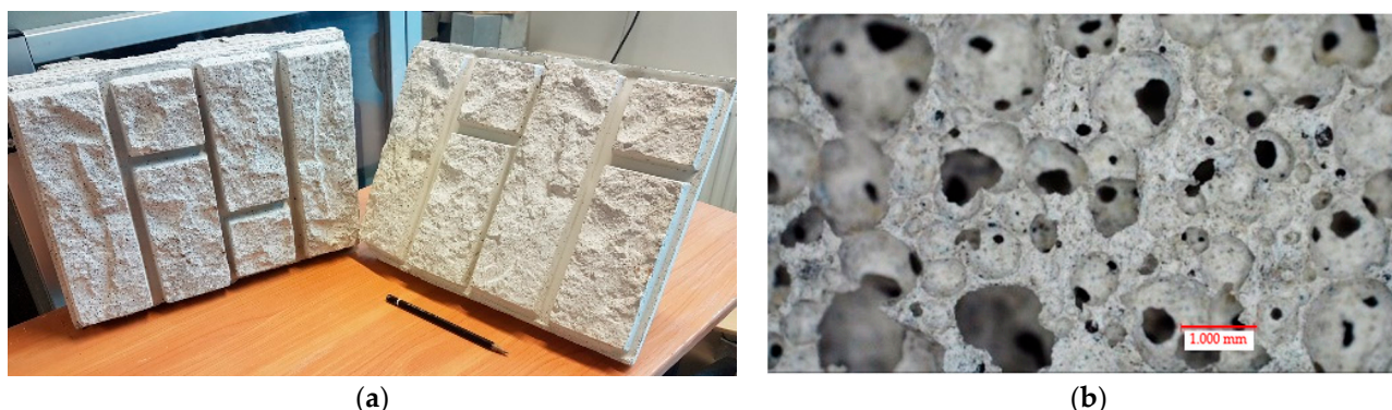
Figure 3. (a) Prototypes of the high-strength ternary system binder's mortar. (b) Foamed and highly porous ternary system binder.
