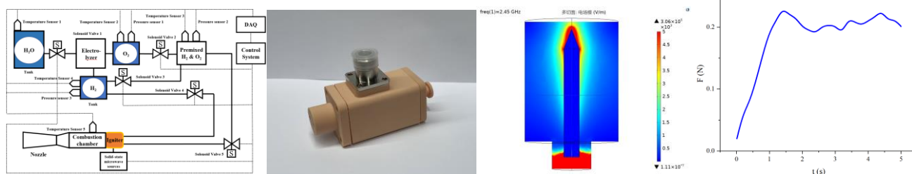
Fig. 1 The microwave water propulsion system integrates modules for electrolyzing water into hydrogen and oxygen gases.
