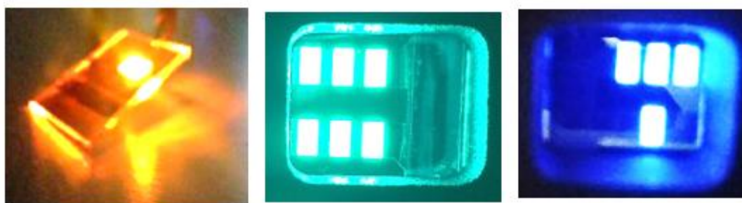
Fig. 1 Two-organic layers OLEDs deposited by solution process (orange-red, green and blue emitters)
