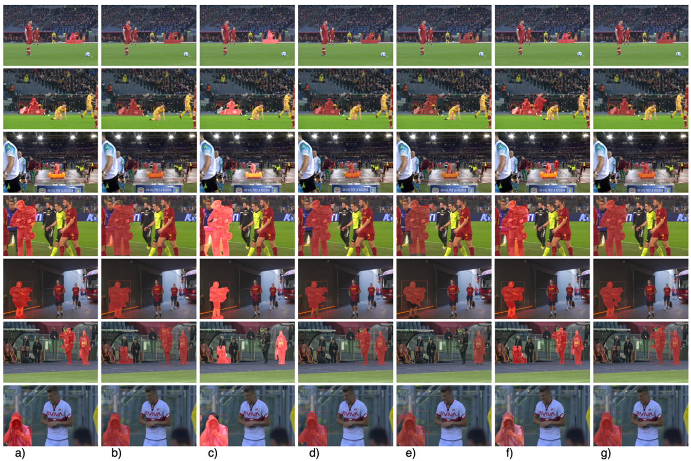
Figure 9. Segmentation results of the compared models for single- and multi-camera operator instances in the aggregated dataset's test images (outlined in red contour): (a) original images with ground truth segmentations; (b) YOLOv5 segmentations; (c) YOLOv6 segmentations; (d) YOLOv7 segmentations; (e) YOLACT segmentations; (f) Mask R-CNN segmentations; (g) YOLOv8 segmentations.
