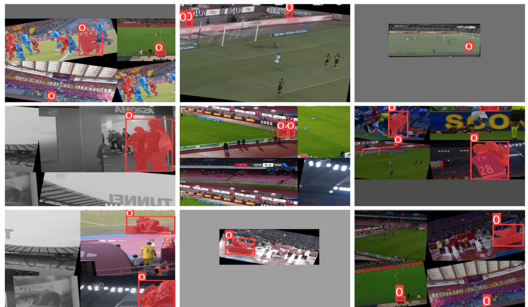
Figure 3. Dataset augmentation. Mosaic, scaling, HSV adjustments, mirroring, and rotation augmentations are demonstrated. Bounding boxes show the instances of cameraman.
