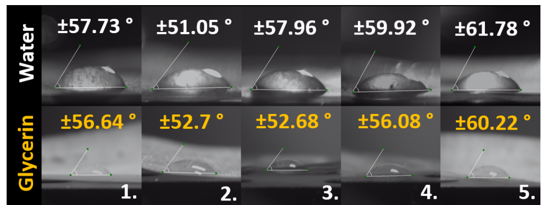
Figure 13. Droplet images and angles of the wettability of coated samples on the solid film mode (1—PVDF/0,05HA, 2—PVDF/0,1HA, 3—PVDF/AgNO 3 , 4—PVDF/HA/AgNO 3 , 5—PVDF).
