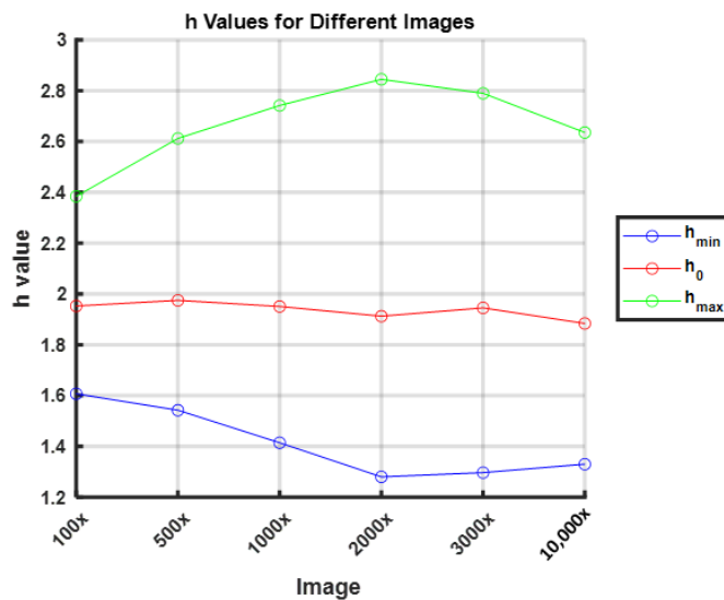
Figure 8. Graphs showing the juxtaposition of three important points on the multifractal spectrum: h_{min} , h_0 , and h_{max} and a graph showing the change in entropy with each magnification: (a) sample a; (b) sample b; (c) sample c; (d) sample d; (e) sample e.
