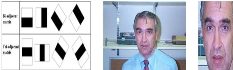
Fig. 4. 5. Face detection features: Rotatable 45-degree (left); Input image (middle); and Face detection outcome (right)
