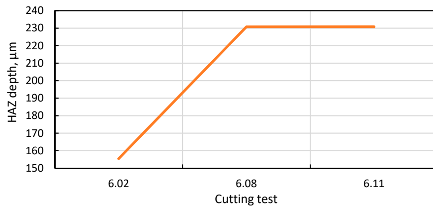
Figure 24. Variation of average HAZ depth of 6 mm thick samples.
