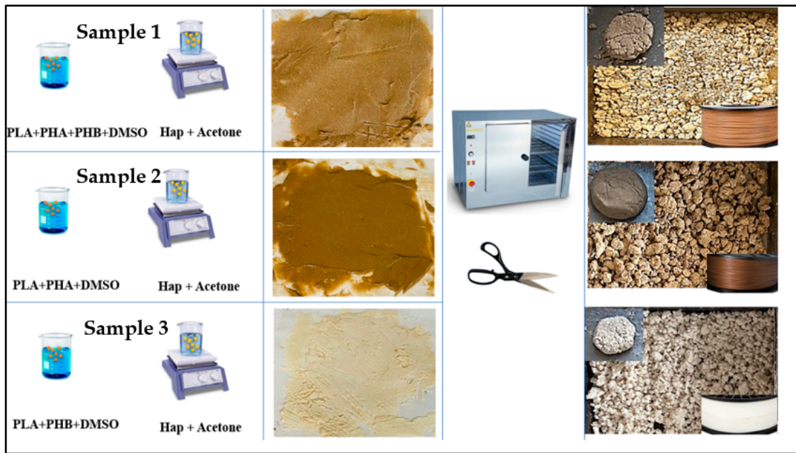
Figure 2. A graphical representation of the PLA/HA/PHB/PHA scaffolds' preparation.
