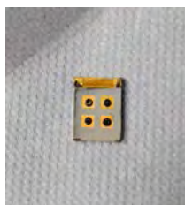
Fig. 1. Sb 2 Se 3 solar cell with Au contacts.
