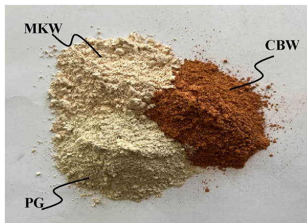
Figure 1. Visualization of the constituent materials: CBW—ceramic brick waste; MKW—metakaolin waste; PG—phosphogypsum.
