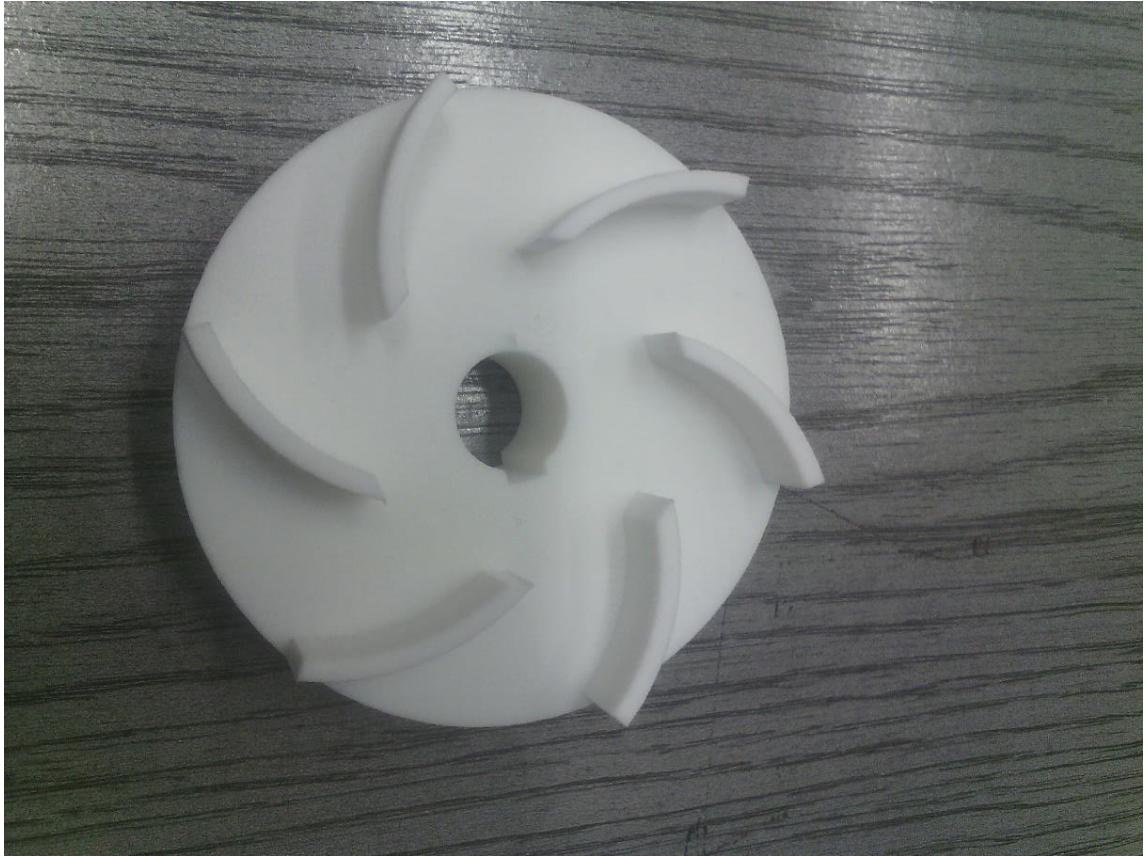
Fig.13.3D printed impeller for sand casting process
