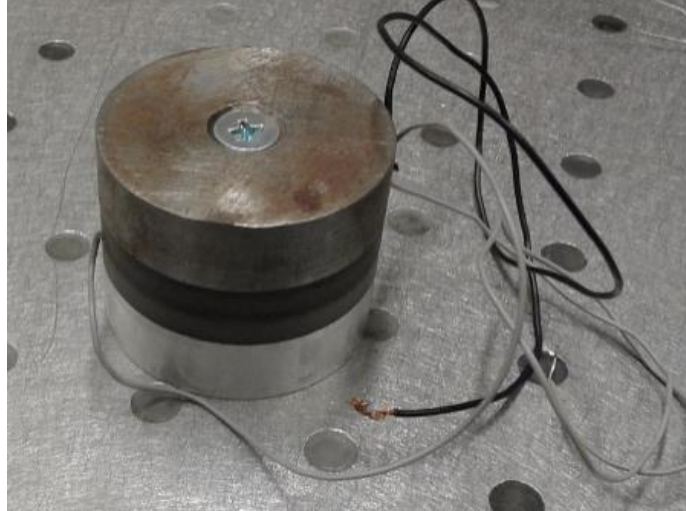
Figure 18. Schematic diagram of vibroactive pad
