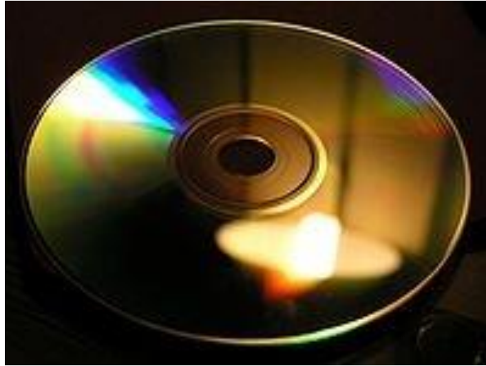
Figure 14. The grooves of a compact disc can act as a grating and produce iridescent reflections[18]
