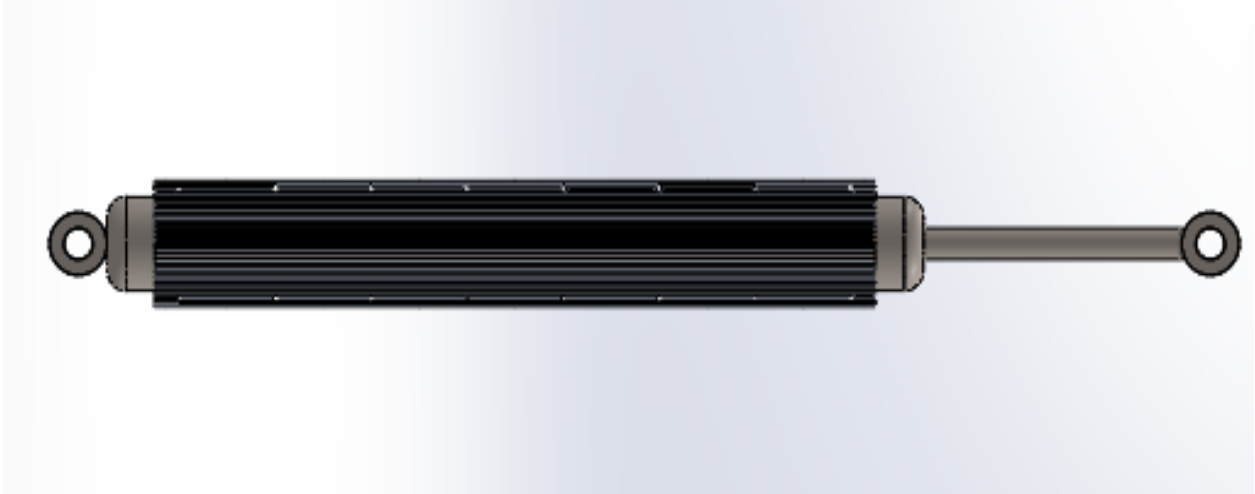
Figure 21: Assembly of hydraulic cylinder with longitudinal fins
