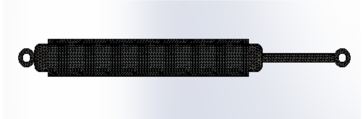
Figure 25: FE Mesh of a hydraulic cylinder with radial fins
