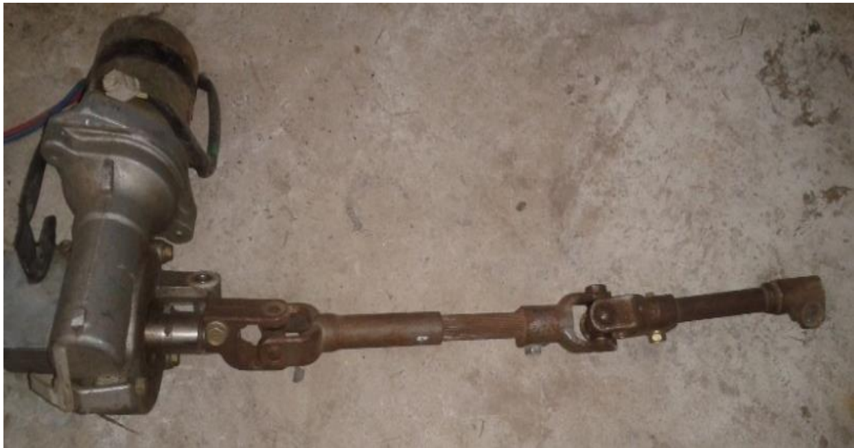
Figure 1: Telescopic splined intermediate steering shaft
