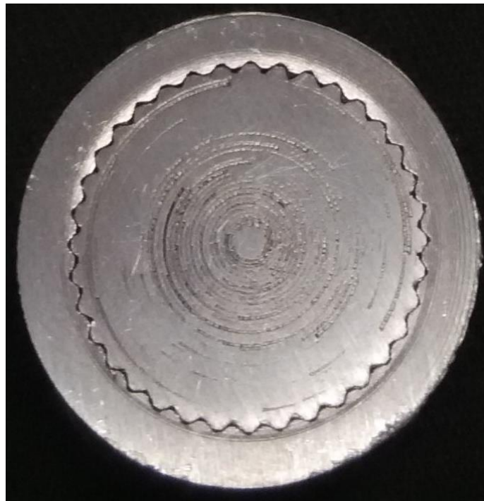
Figure 19: Cross-sectional view of the Spline Shaft
