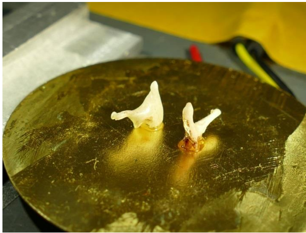
Fig. 2.20 Samples glued on piezoelectric plate
