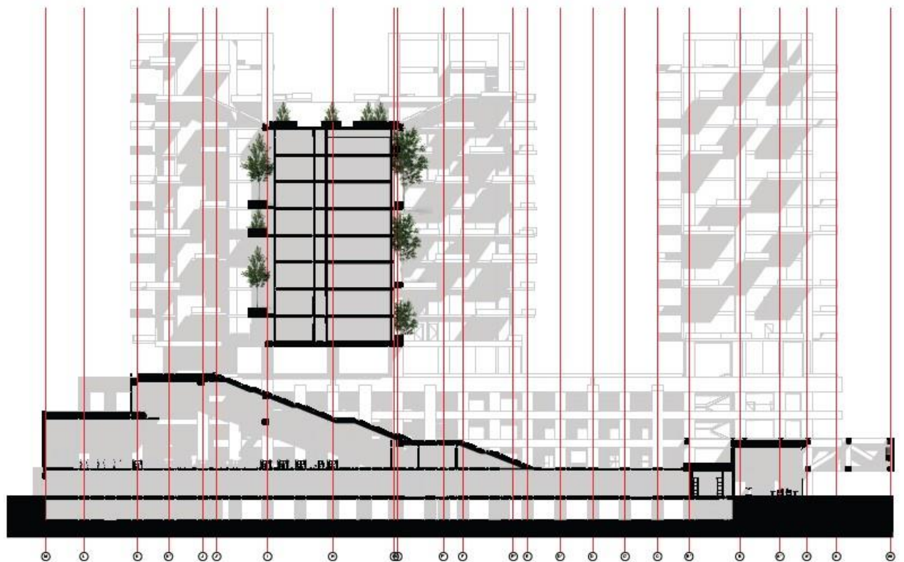
Section S-07. M 1:200. Drawing shows staircase leading to lower park and exhibition hall under them.
