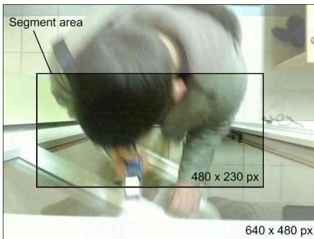
Fig. 4. An example of segmentation is shown. Size and location of a segment should be tuned by context specifics. We placed it in the middle of doors
