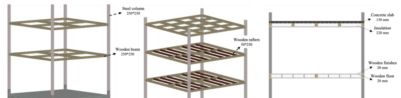
Fig. 67. Steel and wooden foundation with rafters section on upper floors.
