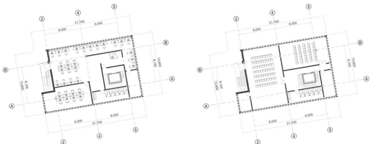
Fig. 61. Third and fourth-floor plan of block B of the multifunctional public library (not in scale) by the author.
