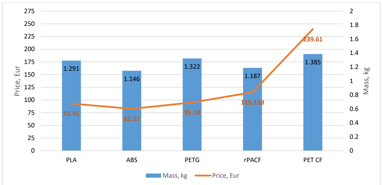
Fig. 25. Dependency between the mass of the exoskeleton's frame and the price of each material
