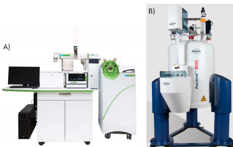
Fig. 7. Autosamplers coupled to analytical devices: A) QS-Works Autosampler by PerkinElmer connected to an LC-MS analytical device [48], B) SampleCase Plus autosampler connected to an Ascend 300 NMR analytical device [49]
