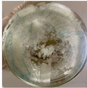
Fig. 16. The appearance of PLA/MCC 2 wt.% composite samples after 24 hours
