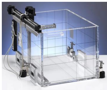
Fig. 17. Water phantom for measuring the distribution of dose [98]
