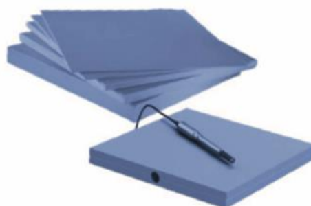
Fig. 18. Solid-state phantoms usually are represented as slab phantoms [101]
