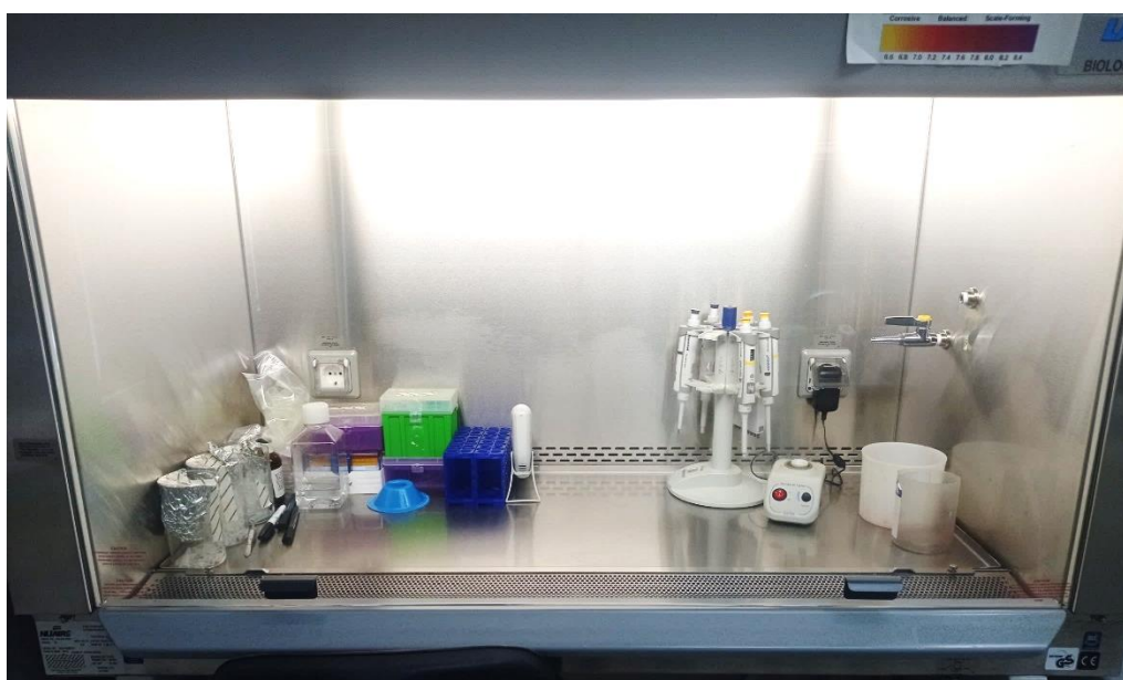
Fig. 9 A laminar flow cabinet at the National Cancer Institute, biomedical physics laboratory
