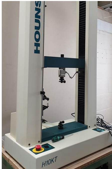
Fig. 17. Tinius Olsen, H10KT universal testing machine [5]
