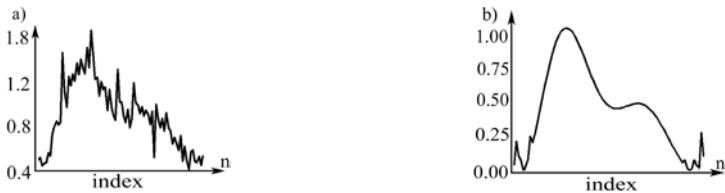
Figure 3.10 Output signal values of the standard PPG (a) and the proposed PPG (b) when SNR= 0dB
