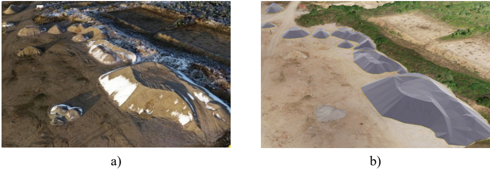
Fig. 16. An example of imported TIN surfaces into photogrammetric software: a) reality mesh in Trimble Stratus platform; b) TIN surface imported into Trimble Stratus software
