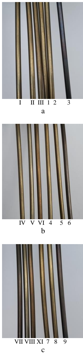
Fig. 8 Variation of oxide film colour of specimens of steel wires tempered in industrial furnace at set temperature 300 °C for 45 min (group A). Numbers below pictures show specimens' numbering according arrangement scheme in furnace (Fig. 3). Approximate colours: a – I, II, 1 and 2 were intense yellow; III was yellow with brown shade; 3 was blue; b – IV, V, 4 and 5 were yellow with different intensity, VI was slight brown; 6 was blue with brown shade; c – VII was brown with blue shade; VIII was intense yellow; XI was intense brown; 7 and 8 were yellow with brown shade; 9 was blue
