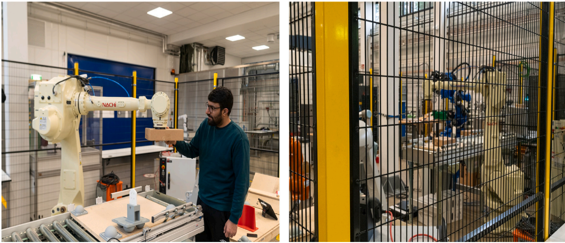
Fig. 3. HRC workspace sharing with human (on left) and conventional robot (on right).
