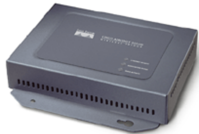
3.2 pav. Cisco Aironet 350 Series prieigos taškas
