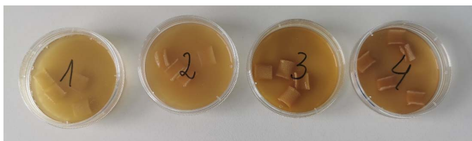
Figure 2. Impregnating liquids with textile samples (Arabic numerals correspond to the sample number).
