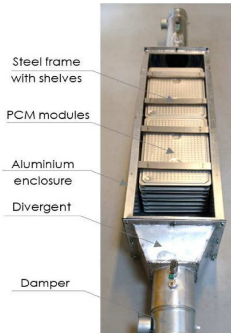
Figure 8. Module arrangement of PCM containment (Zeinelabdein, Omer, and Gan 2018).
