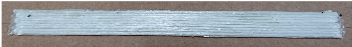
Fig. 1. Photograph of GFRP sample with embedded FBG sensor.
