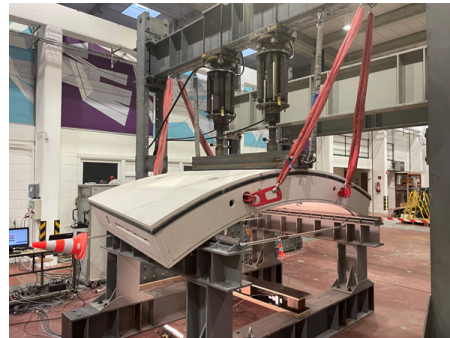
Fig. 3, Full scale 3-point flexural strength test of the tunnel segment
