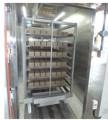
(b) Carbonation curing
