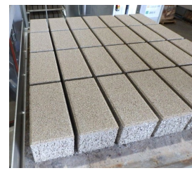
(c) Carbonation-cured low-carbon IL blocks
