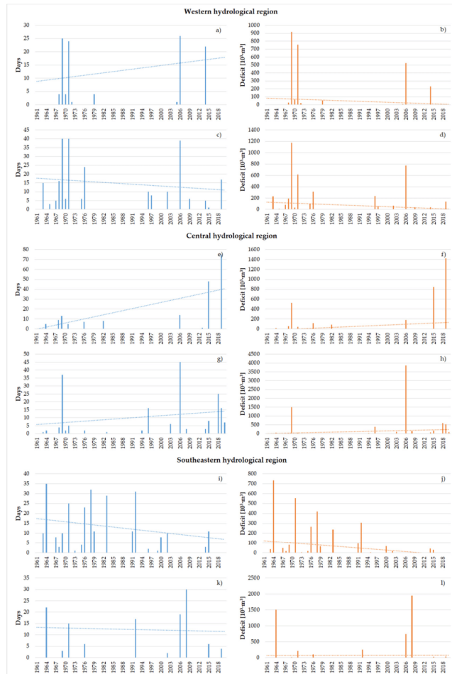
Figure 11. Examples of drought changes for 30Q95 threshold over time: (a) days with drought in JUR river, (b) deficit volume in JUR river, (c) days with drought in MIN river, (d) deficit volume in MIN river, (e) days with drought in SES river, (f) deficit volume in SES river, (g) days with drought in VEN2 river, (h) deficit volume in VEN2 river, (i) days with drought in VER river, (j) deficit volume in VER river, (k) days with drought in ZEI river, (l) deficit volume in ZEI river.
