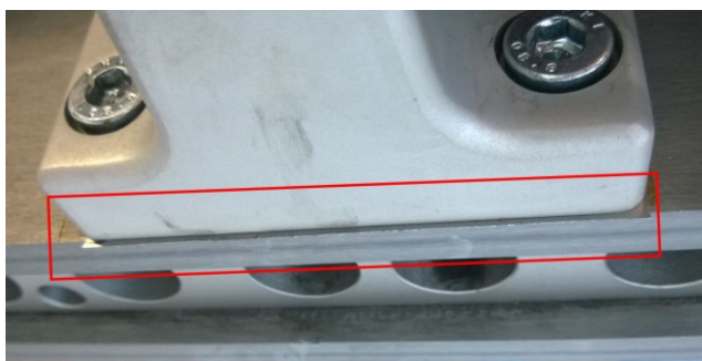
Fig. 21. Metal sheet (0.05 mm) between the upper part of the rotor hub and the rest of the body. This method is used to change the blade angle of attack.
