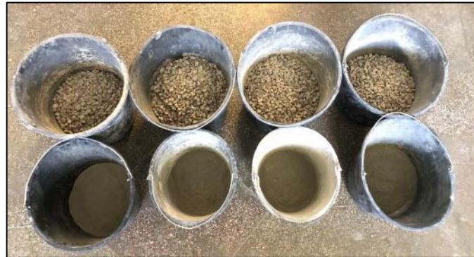
Fig. 12. Materials for batch 01 RCC-W0.30, W0.35, W0.40, W0.45
