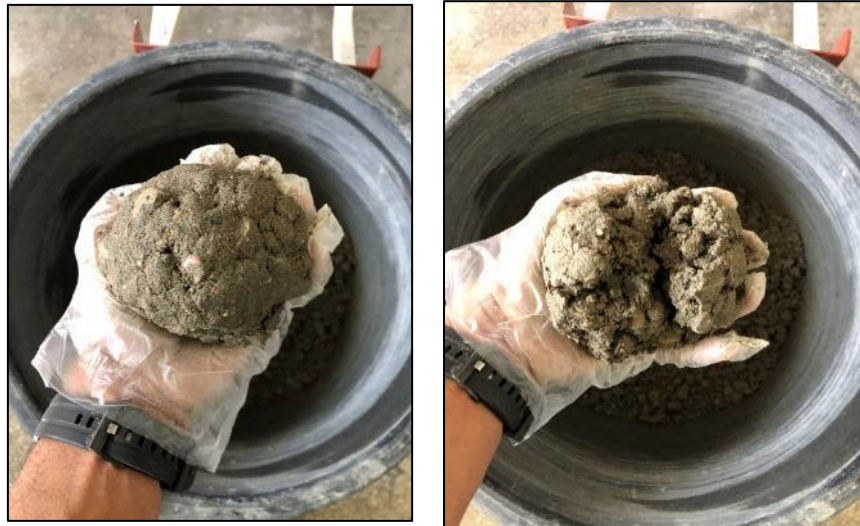
Fig. 25. Flyash content:30% Finger Slump test
