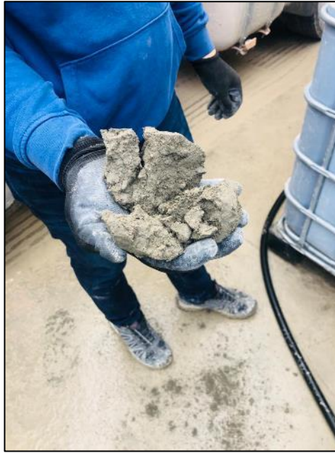
Fig. 49. RCC Snow ball test
