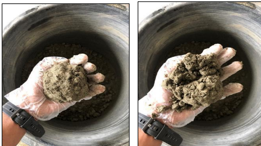
Fig. 17. Sample W/C:0.35 Finger Slump test
