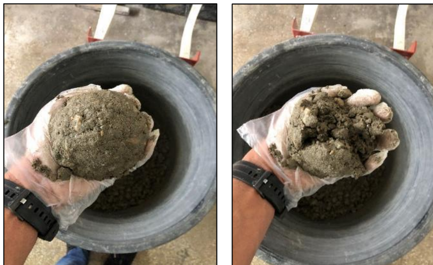
Fig. 24. Flyash content:20% Finger Slump test
