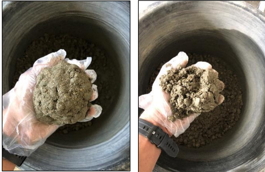
Fig. 18. Sample W/C:0.40 Finger Slump test
