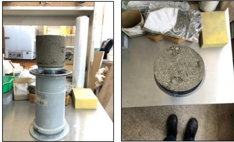
Fig. 30. cement Content 280Kg/m 3 Visual Analysing test
