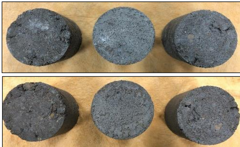
Fig. 44. Set 03, Before & After CDF test
