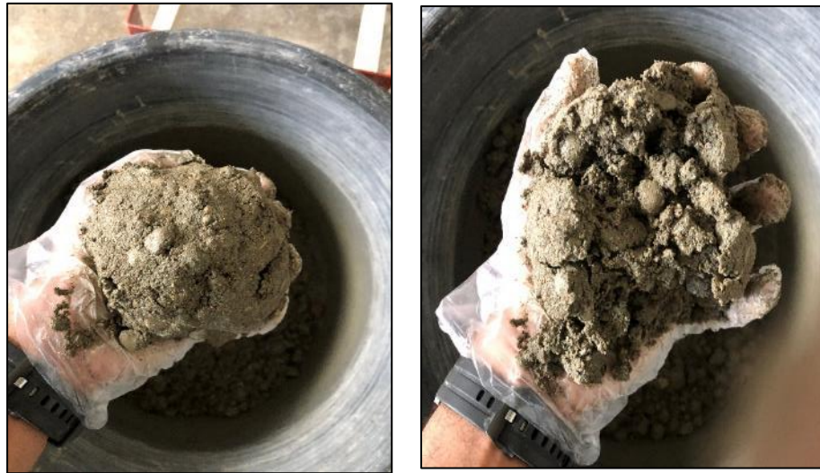
Fig. 23. Flyash content:10% Finger Slump test
