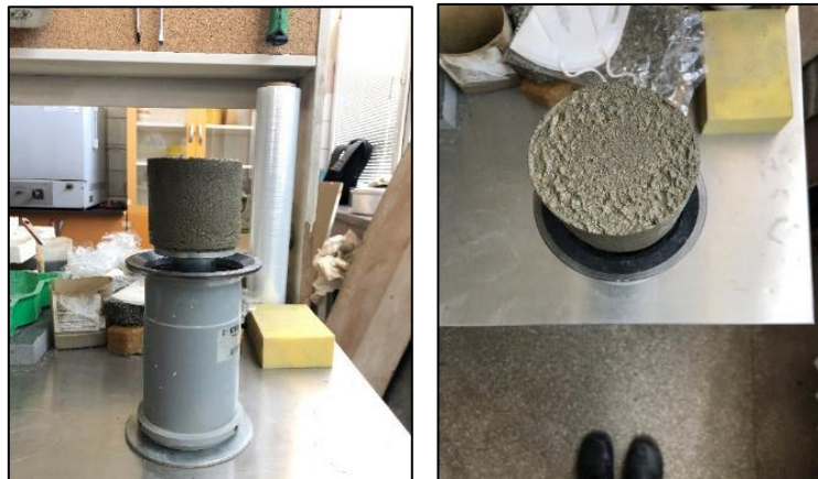
Fig. 31. Cement Content 300Kg/m 3 Visual Analysing test
