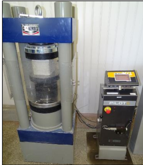
Fig. 5. Compression testing machine Controls 50-C4042, conforming to LST EN 12390-4
