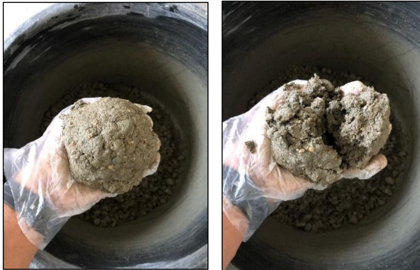
Fig. 21. Cement content:300 Kg/m 3 Finger Slump test
