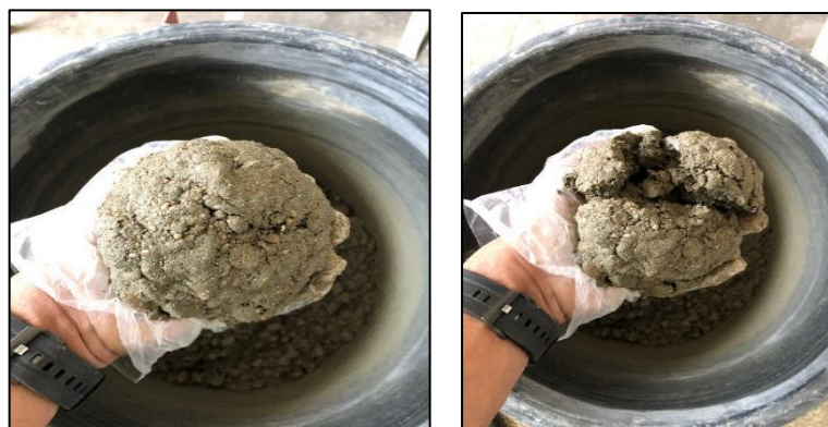
Fig. 22. Cement content:320 Kg/m 3 Finger Slump test
