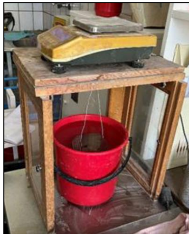
Fig. 40. Water absorption test.
