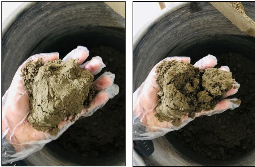
Fig. 16. Sample W/C:0.30 Finger Slump test
