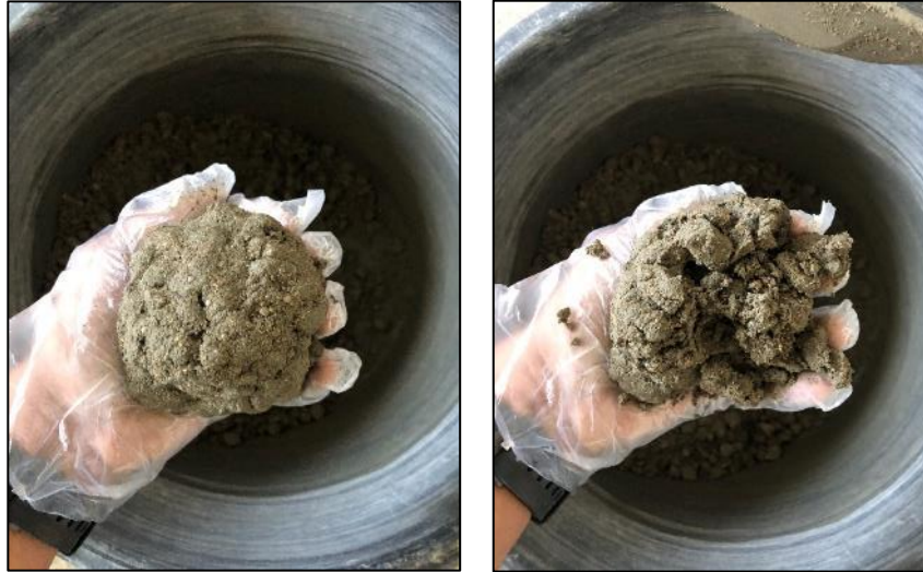
Fig. 20. Cement content:280 Kg/m 3 Finger Slump test
