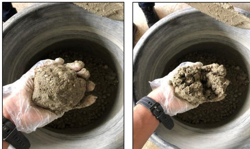
Fig. 19. Sample W/C:0.45 Finger Slump test
