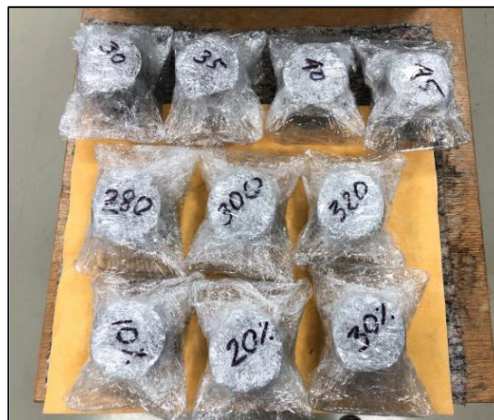
Fig. 41. Specimen wrapped with Nacl Solution for CDF test.
