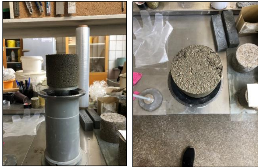
Fig. 33. Fly ash content 10% Visual Analysing test
