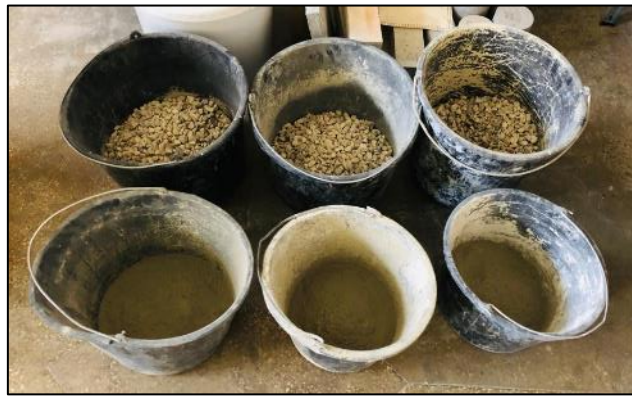
Fig. 13. Materials for batch 02 RCC-C280, C300, C320
